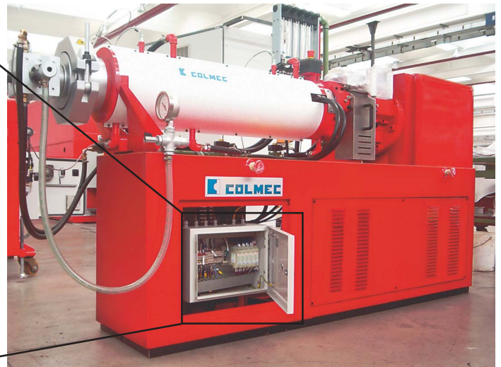
COLMEC extrusion line with Siemens PLC. Control and data acquisition are made by using delatadue series (D1, D8 and D9). A gateway DX 5370 is installed to perform PROFIBUS-Modbus RTU data exchange and manager function for 16 instruments.
